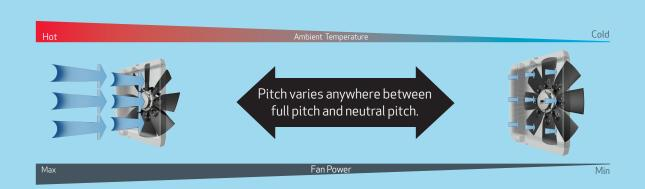
Total Airflow Control (TAC) is AutoReverse and Variable Airflow
